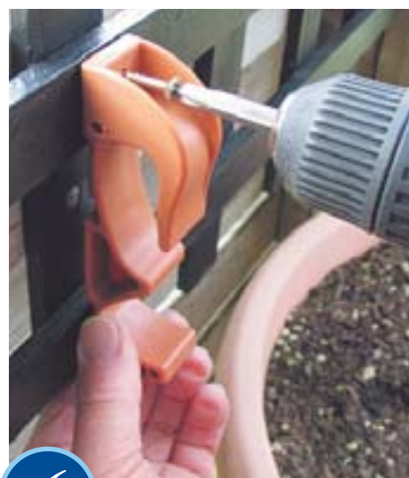
6 FOR bigger, heavier pots, use a specially made pot latch that can be screwed in place. We've used Leyland Latches for our bigger pots.
