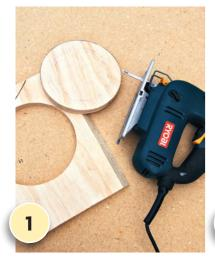
Use a large paint-tin lid and pencil to trace a circle on to a piece of 20mm plywood. Cut out the circle with a jigsaw and smooth rough edges with sandpaper.
