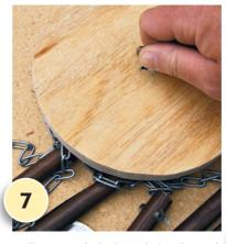
Drill a 3.5mm hole through the plywood circle's centre. Thread the other end of the black nylon cord through, from the underside. Place a blob of PVA glue in the hole and screw the eye-screw in place from the top, as shown. Cut off excess cord.
