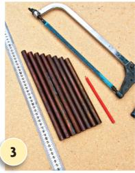
Cut eight lengths of copper piping at differing lengths from 210mm to 280mm, as shown. Smooth rough edges with a metal file.
