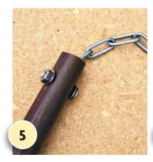
Thread a 4mm bolt through both holes and through the first link of one length of chain. Use a small washer on each side and fix with the nut. Tighten with a screwdriver and adjustable spanner. Repeat with the other lengths of copper piping and chain.
