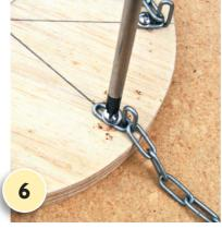
Mark eight equidistant points round the plywood circle. Fix a chain at each point about 15mm from the ply edge with a 15mm screw, as shown. Thread a length of black nylon cord through the sink strainer's central hole and knot it underneath.
