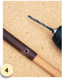
Place the small piece of dowel in the first length of copper piping and drill a 4mm hole about 15mm from the end, right through the piping, as shown. Remove the dowel.
