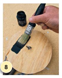
When the glue is dry, apply two coats of Resene Waterborne Woodsman to the plywood circle, allowing each coat two
