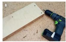
on the space pieces and drill 6 pieces all the way through, with 2 pieces only drilled half way for each end.
