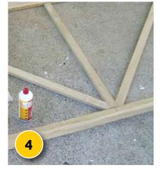
MARK the centre of the main frame, measure and cut the central vertical sunray. Fix with PVA glue and two brass screws, screwed in at right angles into the main frame. Measure and cut the two longest (diagonal) sunrays and fix into position with PVA glue.
