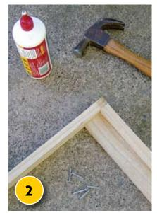
ATTACH the legs to either end of the top horizontal strut for the main frame, using PVA glue and galvanised nails. Repeat for the side frames.
