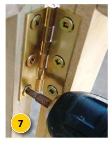
FIX the lower leg struts into position on the legs of the main frame with PVA glue and nails. Attach a side panel to the main panel with two brass hinges. Repeat with the other side panel.
