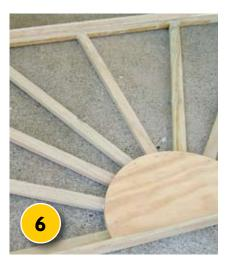
USING the panel pin, string and pen, draw a semi-circle on the piece of plywood. Cut this out with a jigsaw and smooth off any rough edges with sandpaper. Fix the plywood sun into position, attaching it to the frame and each sunray with PVA glue and a nail.
