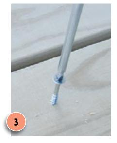
Turn the table the right way up and screw through the pilot holes in the table top, fixing the support braces to the underside of the table top.
