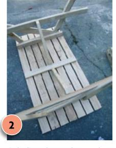
Fix the diagonal support braces to the legs, screwing into position through the pilot holes provided.
