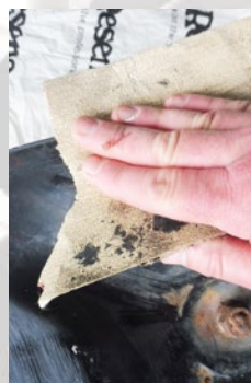
Step three Lightly sand the table top and base to 'key' the surface. Wipe off any sanding residue with a clean cloth.
