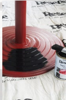
Step seven Apply one coat of Resene Super Gloss to the base and allow to dry.
