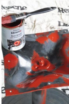
Step five Spot prime any areas of rust or bare metal on the base with one coat of Resene Rust-Arrest and allow to dry.
