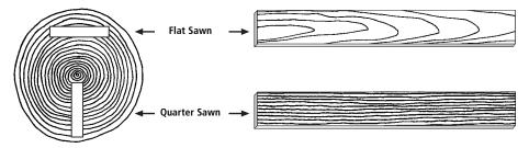
With flat sawn weatherboards and planks, the bark-side will tend to split and crack more than the centre-side.
