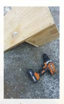
**Step three** Attach the back into position, as shown. Again, fix with PVA glue and 65mm screws, drilling pilot holes first and countersinking the screw heads.
