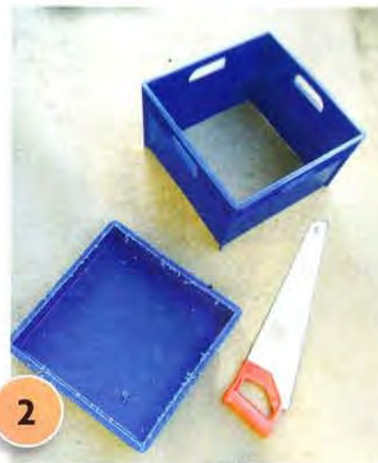
2 Cutting in a straight line, saw the base off one of the plastic storage crates and smooth any rough edges with sandpaper. This sawn-off base will form the top drainage tray of the water feature.
