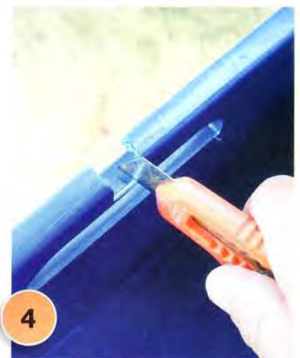
4 Use a craft knife to cut a small notch in the top of the other storage crate, making sure it's large enough to accommodate the power cord of the water pump.
