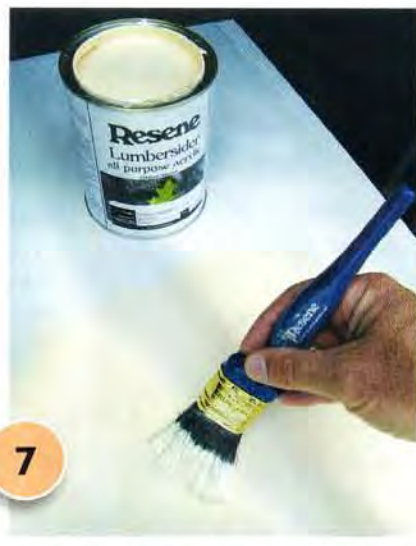
7 Apply two coats of Resene Frangipani to this plywood base, allowing two hours for each coat to dry, then sand the plywood structure in position. Place the larger section of sawn-off storage crate in it and stack the other crate on top.
