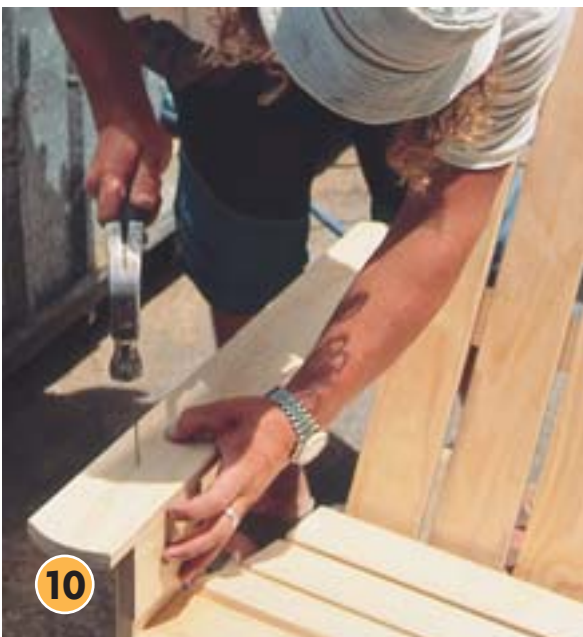
Attach arm rests to arm supports using five 50mm galvanised nails, ensuring you have an 80mm overhang on the front of the chair and the arm rest is flush with the back. The arc detail on the front of the arm rest is optional.
