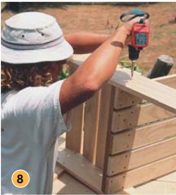
Attach chair back to base legs using three screws on either side. Place the seat at the angle given on the template.
