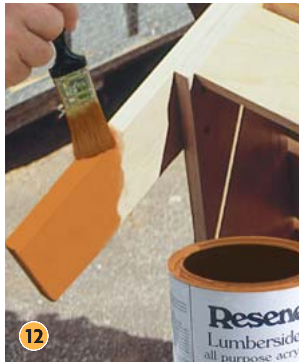
Secure the front seat panel between the front legs using two 60mm galvanised nails at each end, leaving an 18mm gap at the top. Paint chair with two coats of Resene Lumbersider in Resene Hyperactive.
