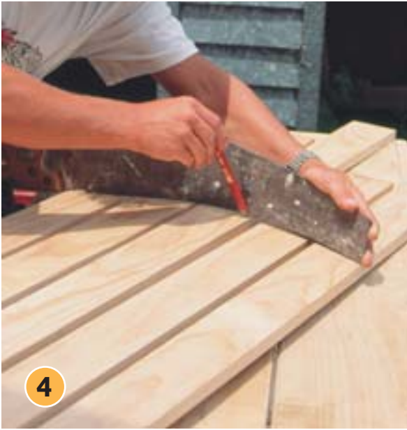
Measure up 750mm from the base of the back on both sides. Mark out an arc between the two points with a bendy piece of thin timber or plastic – we used a saw blade.
