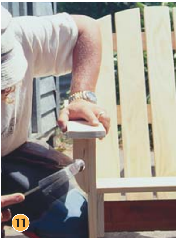
Attach the decorative shaped panels to arm supports and front legs using 50mm galvanised nails.
