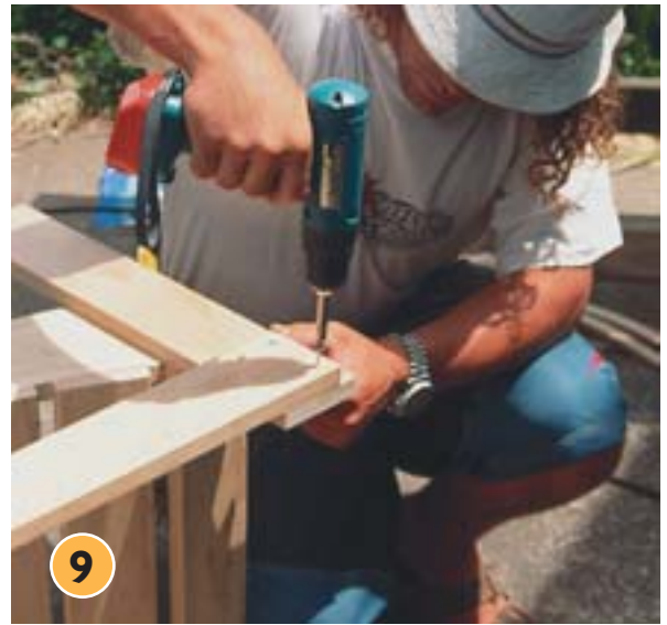
Fix arm rest supports using four screws at each end, ensuring the supports are flush with the top of the front legs but 18mm in to allow for the decorative shaped panel.
