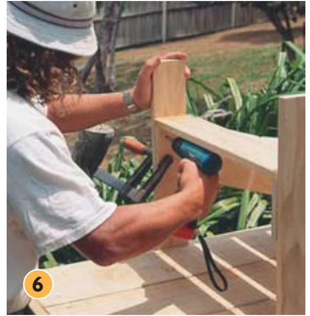
Attach the front legs from the inside of the base legs using four screws at each end. The distance between the underside of the base leg and the bottom of the front legs should be 213mm to ensure the chair sits flat.
