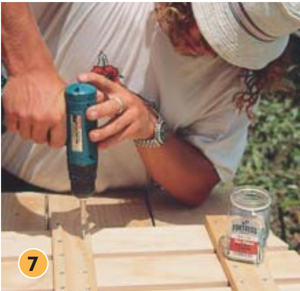
Measure up 380mm from the base of the chair back on the underside to position the middle support. Attach the middle support – the longer of the two back supports – at that mark, ensuring you have an overhang of 36mm on either side to support the arms. Position the top support, ensuring it's flush with the sides. Use four screws per slat.
