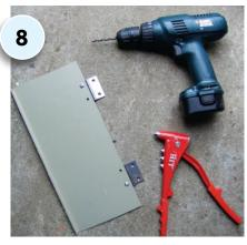
USING a drill and pop riveter, attach the two hinges to the piece of Colorsteel, as shown. Use the masonry drill bit to drill four holes approx 30mm deep, along the upper edge of the back of the mailbox, aligning these holes to the hinges. Attach the hinged flap to the back of the mailbox using the dynabolts and ratchet set.
