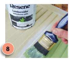
Apply two coats of Resene Chelsea Cucumber to the entire structure. Allow two hours for each coat to dry. Fit the shelves into position on the side supports. Fit the latch or lock.
