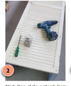
Attach three of the cupboard doors together with PVA glue and screws, as shown, to form the sides and back of the unit.
