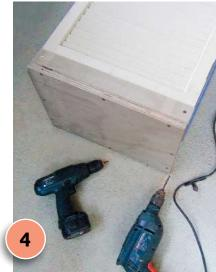
Fix the roof in place with PVA glue and screws. Cut a strip of plywood to fill the space across the unit's back and front (this isn't necessary if your doors are the same height). Fix the unit's door in place with the hinges and screws.
