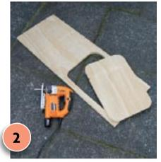
With the jigsaw, cut a hole in piece A for the sink, as shown. Smooth rough edges with sandpaper.
