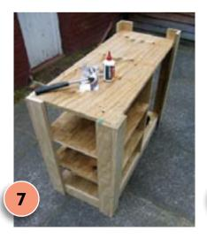
Turn the unit upside down. For the base, glue and nail piece B into place. Use zinc-plated screws to attach three castors along B's shortest edge so the unit stands level when up the right way.
