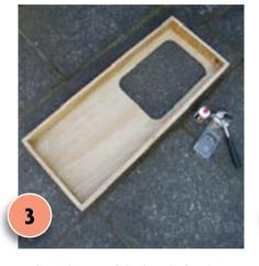
To form the top of the bench, fix pieces C and D to piece A with nails and PVA glue.
