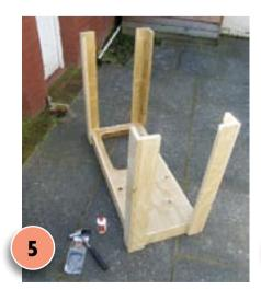
Turn the top upside down. Nail and glue the two longer legs to one end of the bench. Then nail and glue the two shorter legs to the other end. Use a set square to ensure the legs are at right angles.
