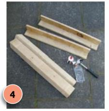
To form the legs, fix pieces E and F together, and pieces G and H together, with nails and glue.
