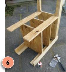
Turn the unit on its side. With PVA glue and nails, fix pieces J to pieces I to form the shelves (check they are level and evenly spaced).
