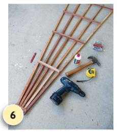
Measure, mark and fix the three remaining crosspieces, ensuring they are evenly spaced. Allow glue to dry.
