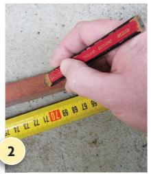
Measure across the top and bottom of the fan shape and measure and mark cross-pieces to fit (ours measured about 700mm)
