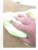
**Step four** Wipe off any sanding residue with a clean cloth.
