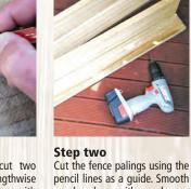
pencil lines as a guide. Smooth rough edges with sandpaper. Attach two 800mm (full width) lengths to two 800mm (half width) lengths at right angles, as shown, fixing securely with 65mm screws and PVA glue.
