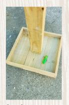
**Step 6** Position the remaining piece of timber in the centre of the table top, as shown, and fix from underneath with screws driven in at an angle.
