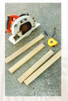
**Step 4** From the 50mm x 25mm timber, measure, mark and cut two lengths at 470mm and two lengths at 410mm. Smooth any rough edges with sandpaper.
