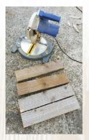
Step 2 Take two of the larger sections of wood and cut into four 450mm lengths to form the table legs.
