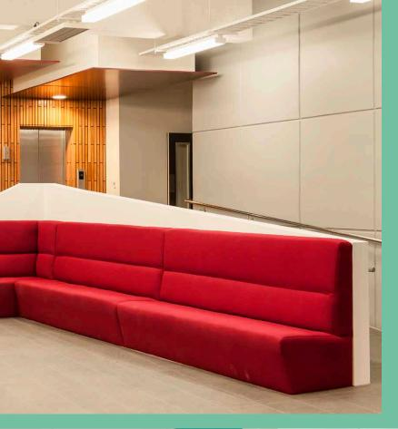
with Resene to develop a suitable specification that could be rolled in-situ. Resene Lustacryl semi-gloss waterborne enamel was selected in vibrant shades of red and burgundy (Resene Livewire, Resene X Factor, Resene Breakfree and Resene Courage). General interior areas are finished in Resene Wan White with doors and exposed steelwork in Resene Fuscous Grey.
